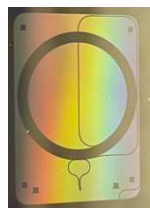
Photo of multi-turn waveguide on silicon nitride chip (radius = 6.1 mm)
